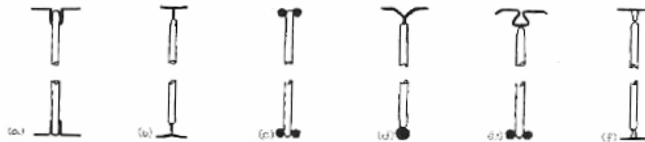
(c) SECTION THRU JOISTS SHOWING FLANGE TYPES
